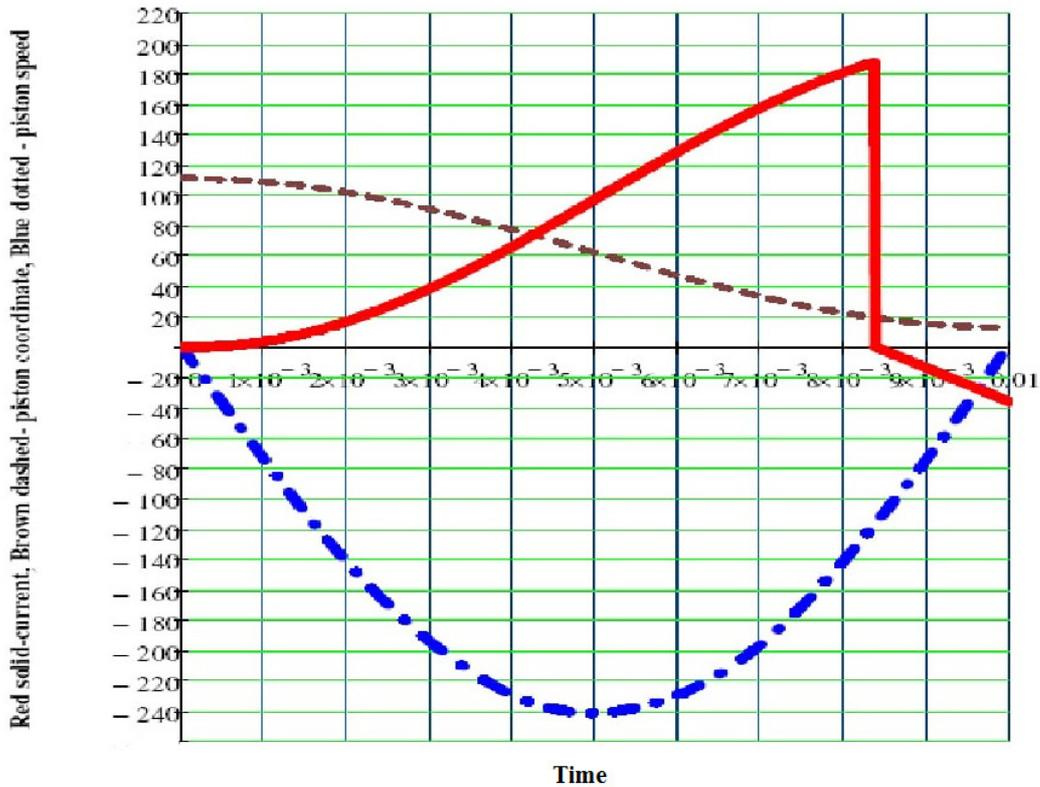
Fig. 4. Piston movement, piston speed and generator current in one cylinder of engine – generator model with auxiliary electric drive
