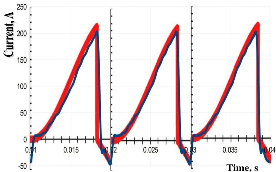
Fig. 6. **Comparison of recorded induced current (blue line) to theoretically modelled current (red line)**
